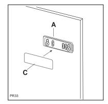
Open the appliance door and the furniture door at 90°. Insert the small square (B) into guide (A). Put together the appliance door and the furniture door and mark the holes as indicated in the figure. Remove the squares and drill holes with Ø 2 mm at 8 mm from the outer edge of the door. Place the small square on the guide again and fix it with the screws supplied.
